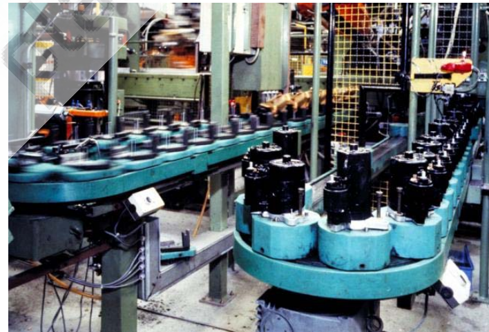
Fig. 4.j. Starter Motor Assembly Conveyor
