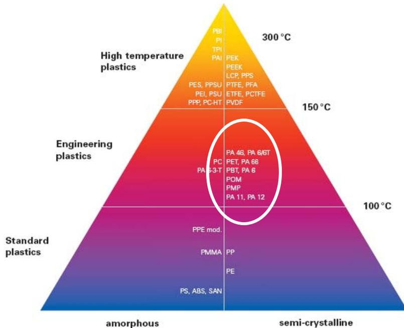
Fig.1. Thermoplastic Pyramid
