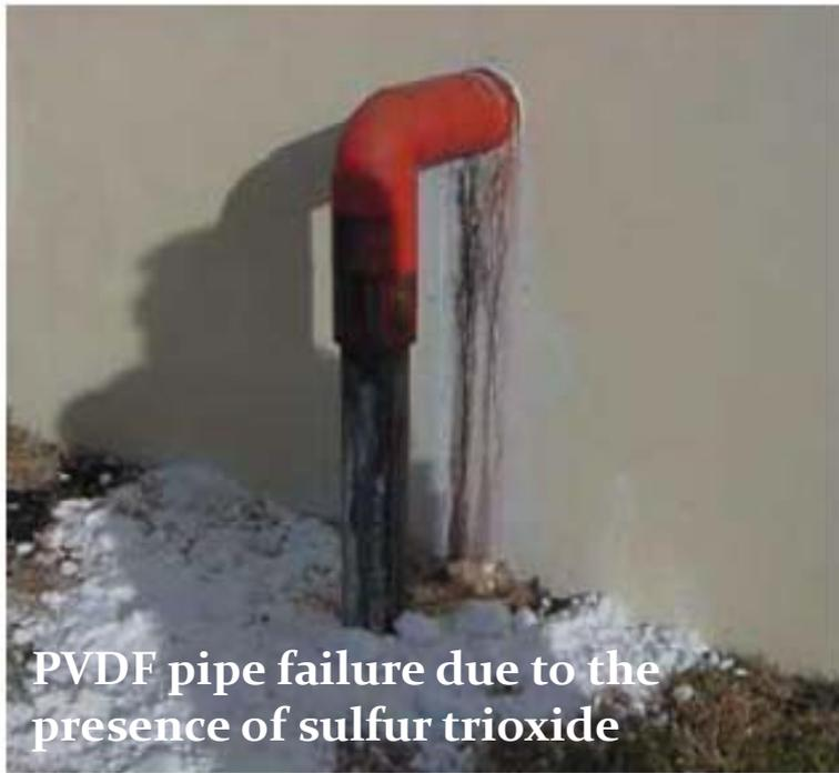
PVDF pipe failure due to the presence of sulfur trioxide
